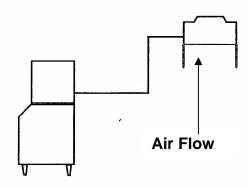
DO NOT Install any part of the refrigerant lines below the quick connect fittings at rear of machine.
